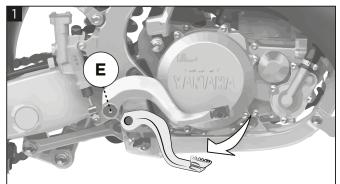
To mount the X-Power cluthc cover, begin by unscrewing the brake pedal bolt (E).
