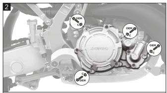
Remove the four OEM clutch cover bolts as indicated in the image. Attach the X-Power cover (A) using the four OEM bolts and four bushings (C). Torque the bolts to the OEM suggested torque settings as indicated in your owner's manual. Then, re-connect the rear brake pedal by re-inserting the brake pedal bolt (E) and then torque to the OEM suggested torque settings as indicated in you owner's manual.
